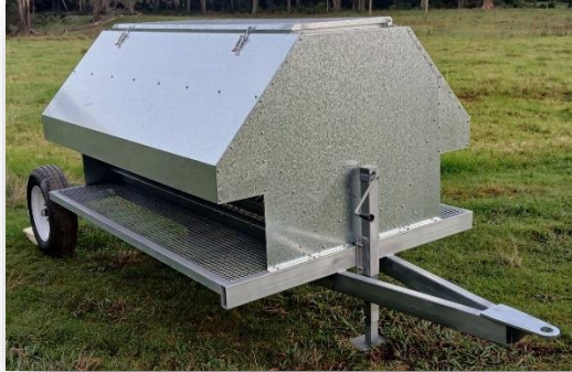
• Figure 5.6.2, Figure 5.6.3 Feed and Water Trailers: Compact, covered trailers stationed adjacent to each caravan, supplying feed (approx. 0.115 kg/hen/day) and potable water. These trailers are mobile and replenished as needed, eliminating the need for fixed external feed or water storage sheds elsewhere on the property.
