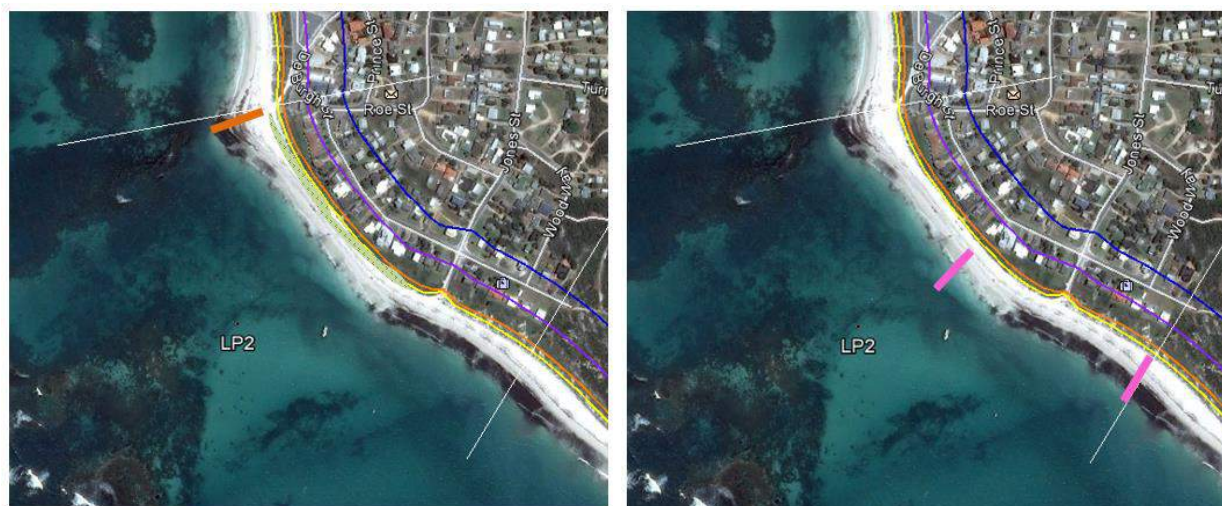
Figure 5-4 Conceptual representation of existing groyne refurbishment and extension, with sand nourishment and potential locations for future groynes
