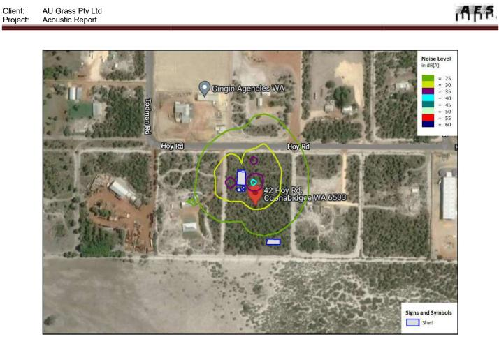
Figure 6: Worst-case noise level contours for scenario 1.
