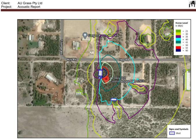
Figure 7: Worst-case noise level contours for scenario 2.
