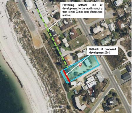
Figure 2: Alignment of proposed development in comparison to its surroundings
