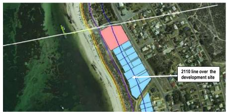
Figure 3: Excerpt from Shire of Gingin CHRMAP with the blue line showing the coastal hazard line at 2110. The proposed development is almost entirely located forward of that hazard line.
