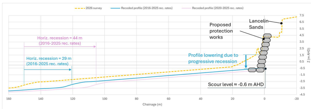
Figure 20. Profile recession and scour level.
