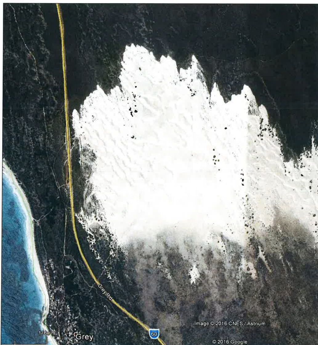
Figure 36. Grey Dune showing proximity to Indian Ocean Drive and general direction of migration towards the north-northwest. Note that western 350m width of the dune is heading towards intersecting the highway. Map data: Google, © 2015 CNES/Astrium.
