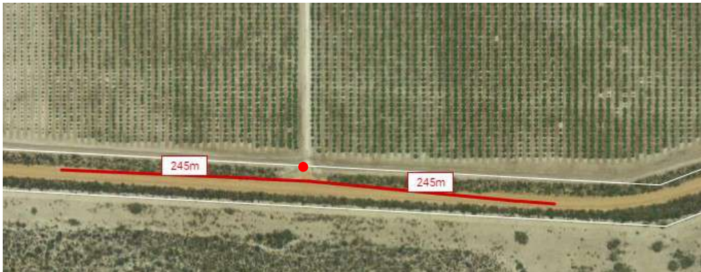
Figure 5.7a: Desirable Sight Distance (say 100km/h) to the west and east of Existing Main Site Access
