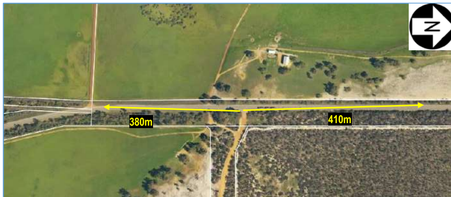
Figure 9: Sight Distance Measurement at Aurisch Road / Brand Highway Intersection
