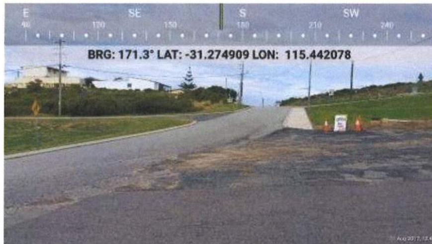
Photo Point 3: Low threat road verge and non-vegetated road excluded from classification under Clauses 2.2.3.2 (e) and (f) of AS 3959, Class D scrub in background (left), Class C shrubland in background (right).
